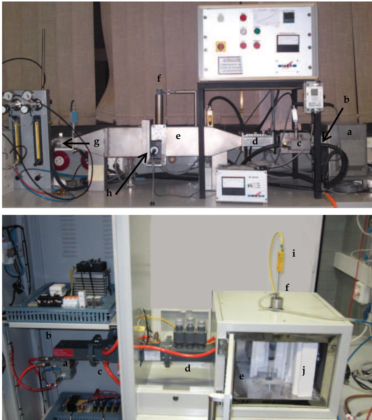
Fig. 1. Photographs of singlemode (upper) and multimode (lower) microwave ovens at INCAR ( www.incar.csic.es ) showing: a) magnetron; b) waveguide; c) circulator with reflected power meter; d) tuning screws; e) resonant cavity; f) reactor; g) terminator with transmitted power meter; h) infrared optical pyrometer; i) thermocouple; and j) insulating material
