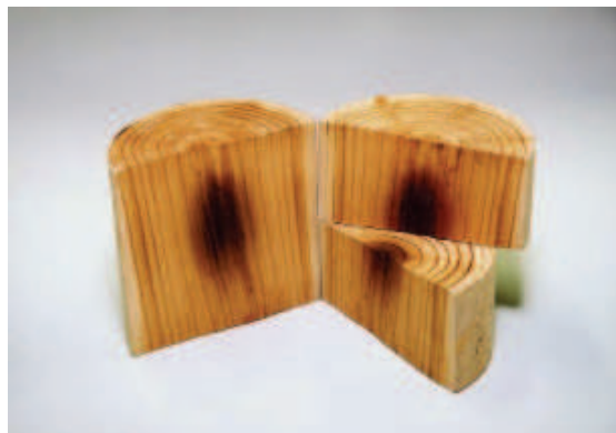
Fig. 5. Cross-section of wood after 3 minutes of microwave radiation (Reprinted from Miura et al., 2004, with permission from Elsevier)
