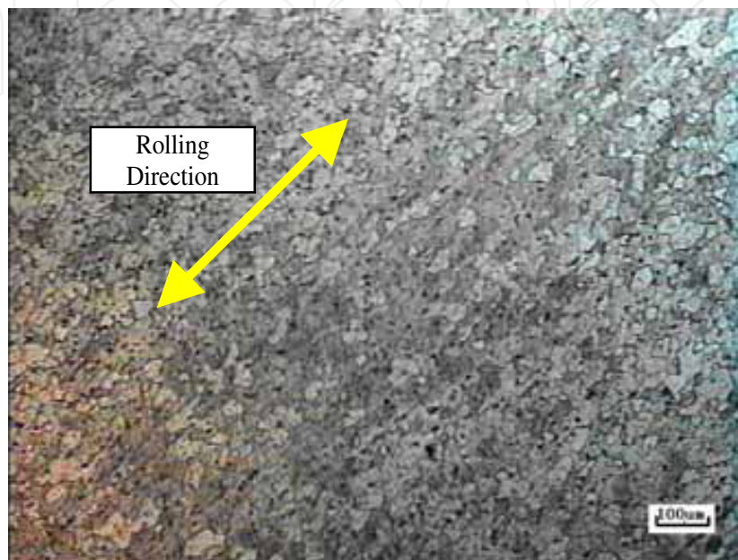
Fig. 6. Microstructure of rolling plate 5052H34
