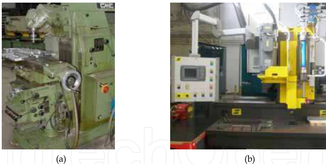
Fig. 8. FSW equipments used to produce FSW samples. a) Conventional milling machine and the ESAB LEGIO™ FSW 3UL.
