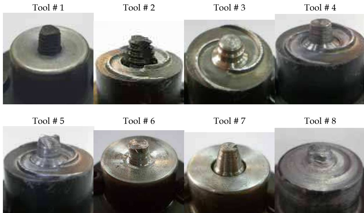
Fig. 9. FSW tools used to produce defect and non defect condition on AA2024-T4 and AA5083-H111
