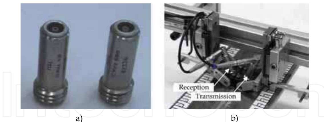
Fig. 19. ToFD ultra-sound NDT testing of AA5083-H111. a) 15 MHz ToFD probes used, b) Arrangement of the probes and motion device.
