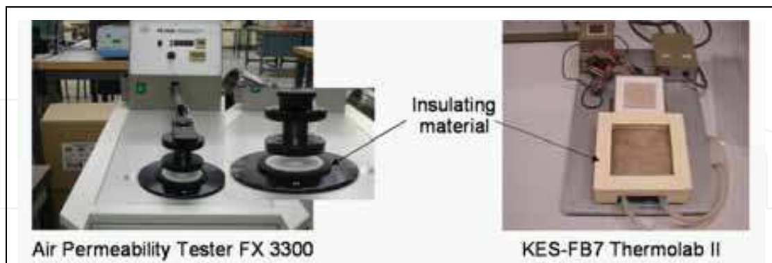
Fig. 18. Customization of testing apparatus for air permeability and thermal conductivity
