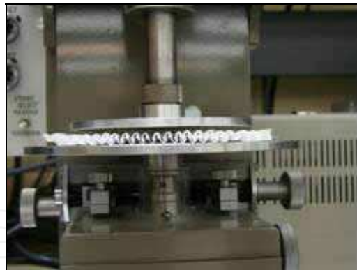
Fig. 20. Customization of the KES-FB3 compression tester
