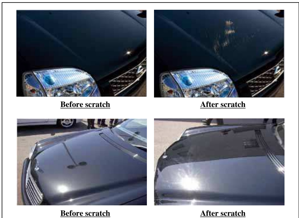
Fig. 4. Visual differences of automotive coating before and after scratching.
