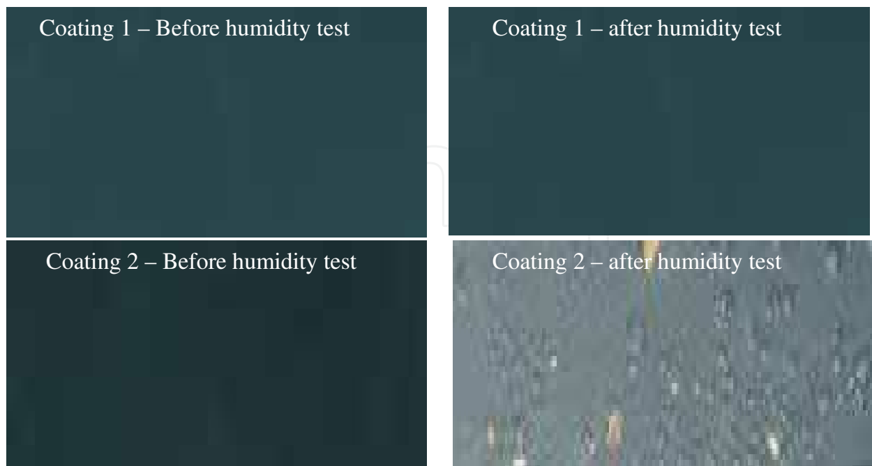
Fig. 12. Results of humidity test for different types of coating.
