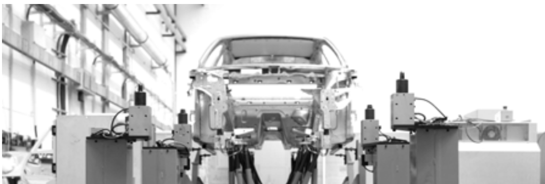
Fig. 4. Car body on track motion carried by flexible positioners (background) and flexible positioners taking over the car body in the next cell (foreground)
