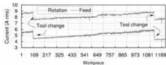
Fig. 3. Evolution of the tool wear using the electrical power consumption.
