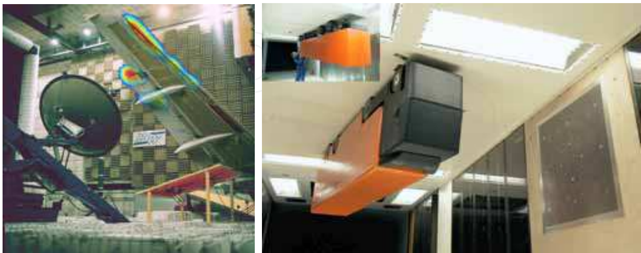
Fig. 12. Test setup examples: full-scale wing in the LLF (left) and scaled truck model in the LST (right)
