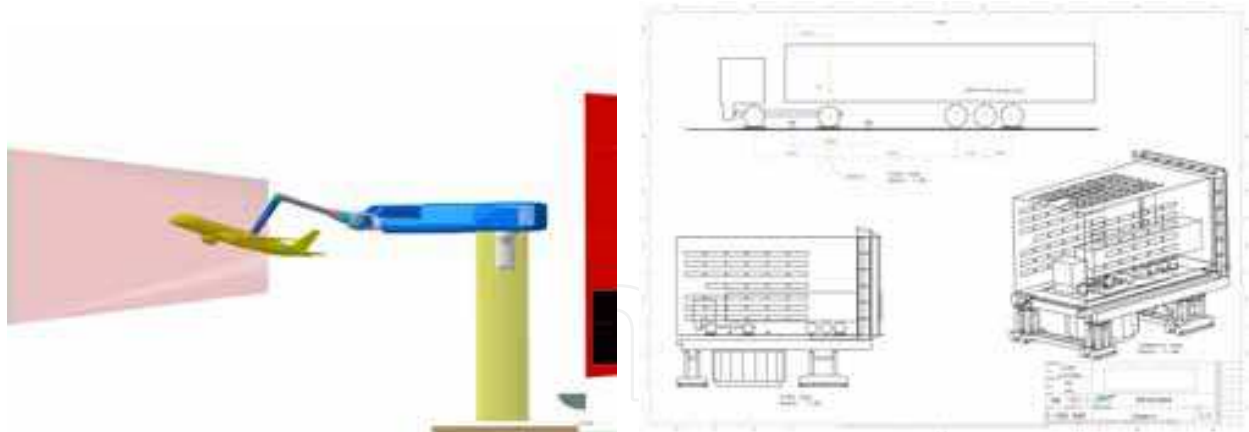
Fig. 5. Sting support system (left) and truck setup in the 9.5x9.5 test section (right)
