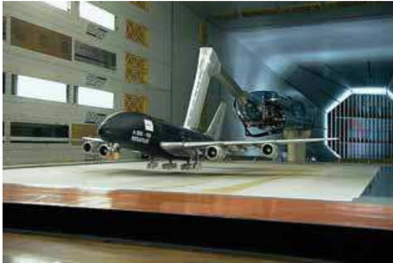
Fig. 6. Model on sting above moving belt
