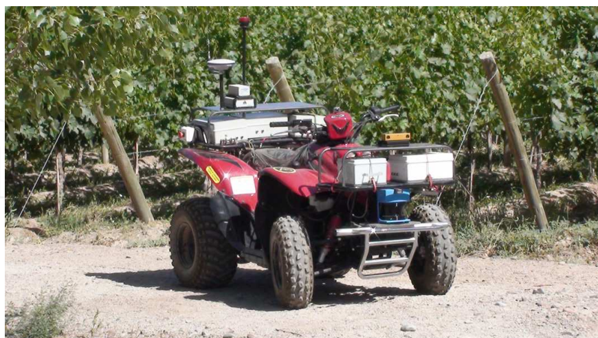
Fig. 1. Prototype of a UGV equipped with a number of sensors. This prototype belongs to the Instituto the Automática of the Universidad Nacional de San Juan.
