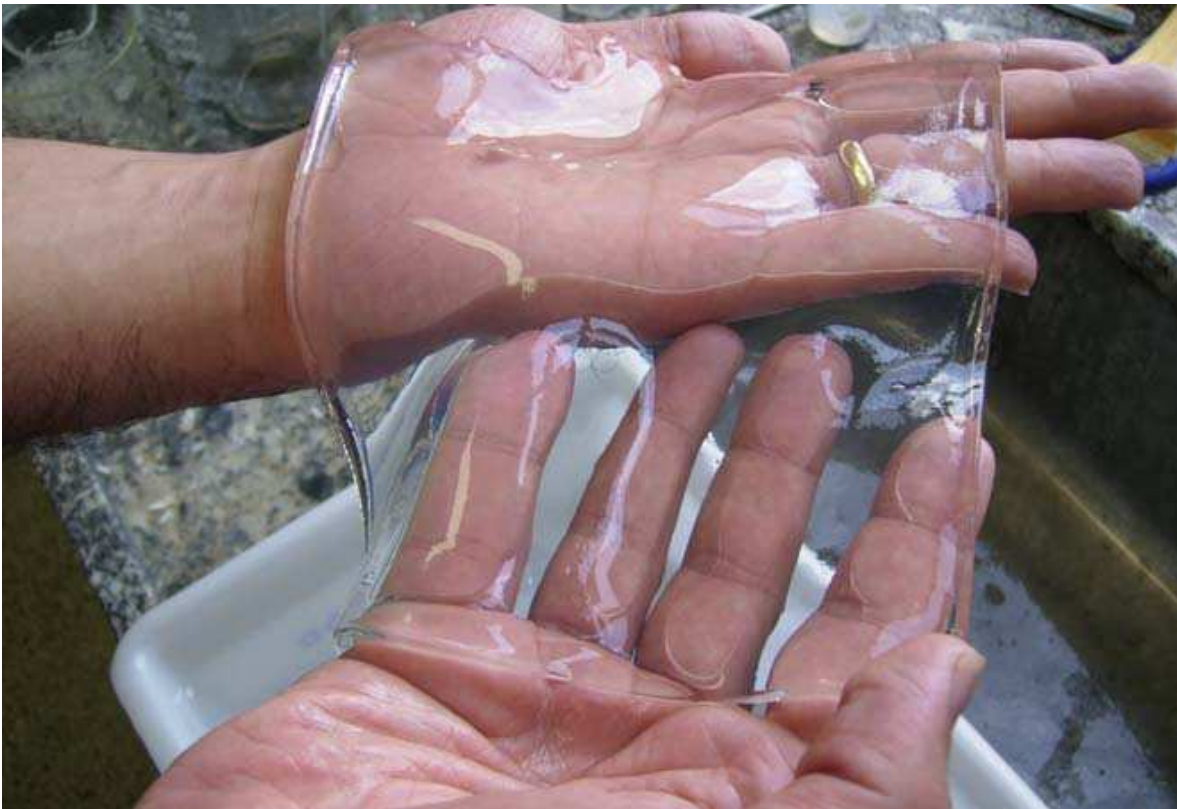
Scheme 1. Photo of hydrogel composed of PAAm and MC in membrane form after dialysis process: [AAm] = 6.0 in w:v%; [MC] = 1.0 in w:v% [Aouada et al., 2010].
