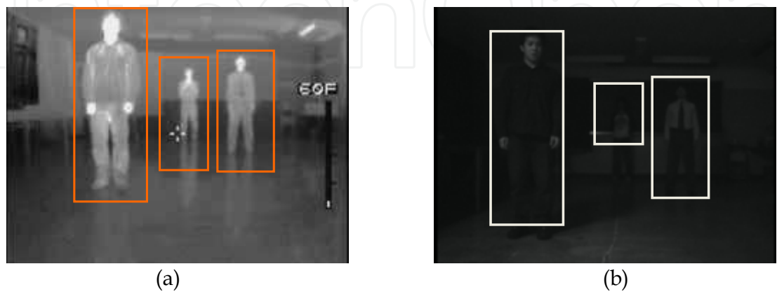
Fig. 22. Outdoor scene illustrating pedestrian extraction: (a, b) representation of the blob detected for both IR and visible images
