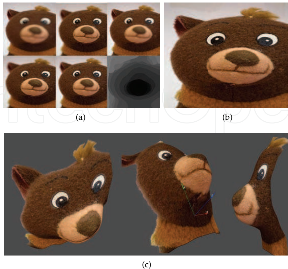
Fig. 11. (a) A few samples of blurry images with height map, (b) finally fused image, (c) reconstructed 3D model.
