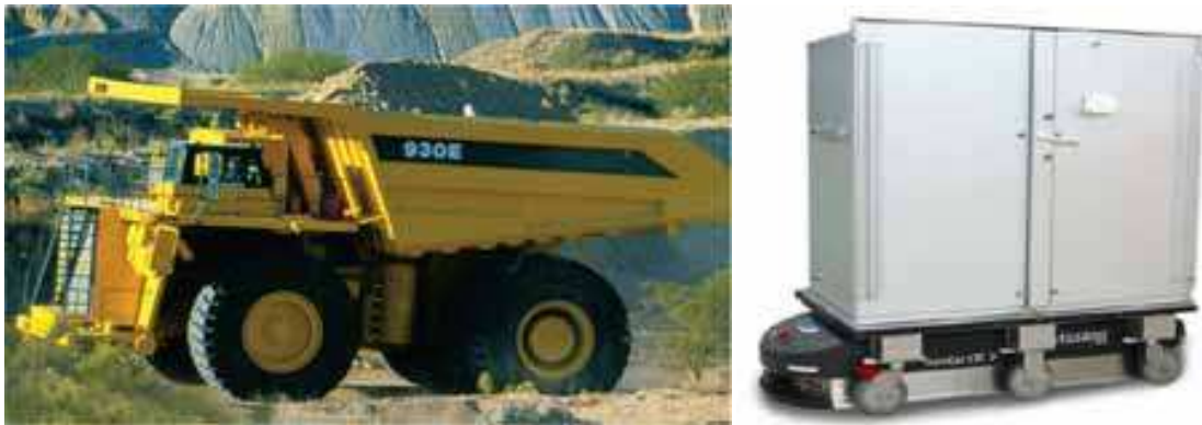
Fig. 1. Two examples of ATS: the automatic hauler truck Front Runner from Kumatsu operating in outdoor, and the autonomous trailer drive from Swisslog operating indoor.
