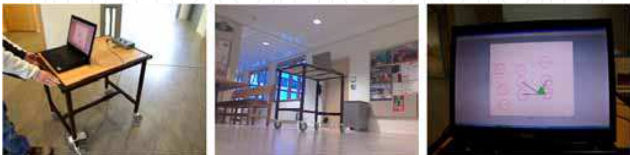
Fig. 20. Simultaneous localization and map building using only visual information at MDH. The table was moved at about 1m/ s producing the map of the room with 9 landmarks on a surface of about 50 m 2
