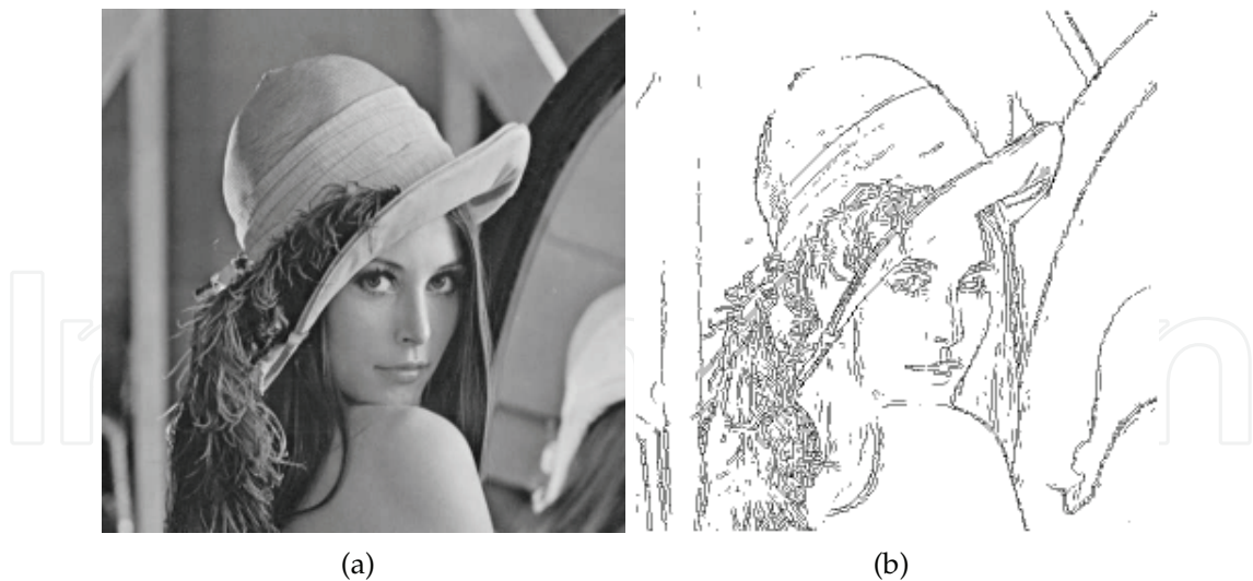
Fig. 9. a) Input image ( Lenna ). b) Edges detected using the MRF model in (Tardón et al., 2006).
