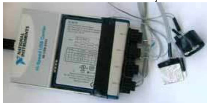
Detail of NI 9219 with sensors
