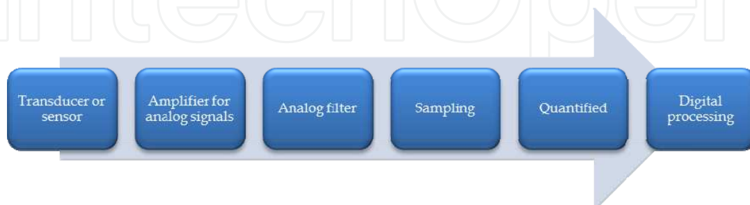
Fig. 6. General block diagram of a procedure analogue to digital (Bronzino, 1999)
