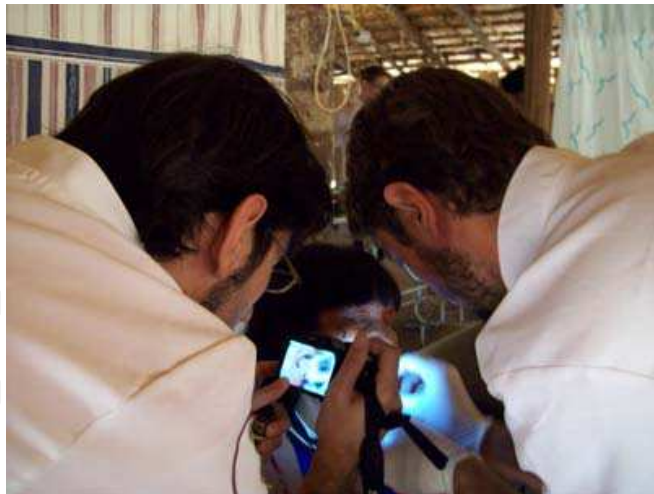
Fig. 2. Image acquisition of patient lesion using illuminator prototype attached to a Sony digital camera
