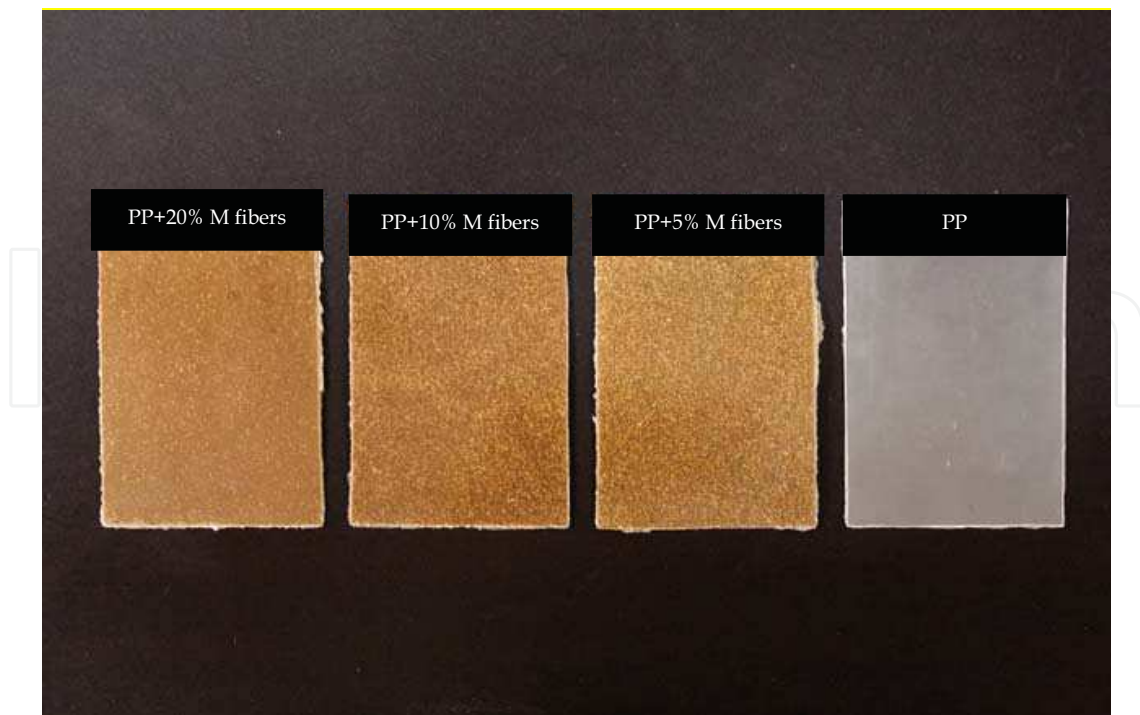
Fig. 4. Biodegradable flax composites made of polypropylene (PP) enriched with different content of bioplastic flax fibres (M plants). The control composite is made of polypropylene with no addition of flax fibres
