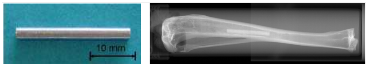
Fig. 1. Implant material and implant location: extruded magnesium pin (a) and radiographical picture of the implant location in the rabbit tibia (b)
