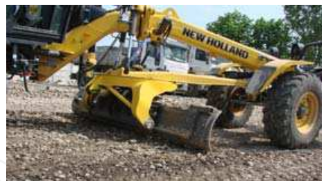
Fig. 3. Laser controlled electro hydraulic leveling machine (courtesy New Holland)
