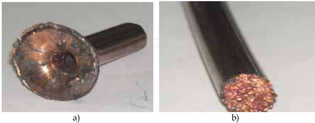
Fig. 3.8. The flow-through flaw on after end (a) and loosening on exposed face (b) of samples obtained from fibrous pressing
