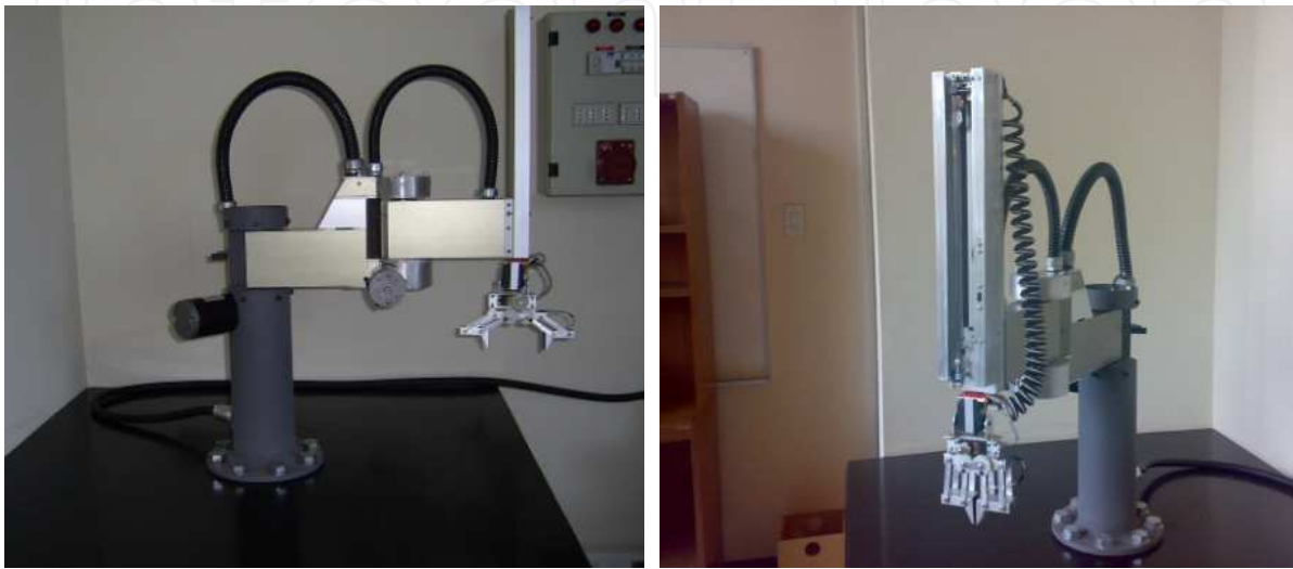
Fig. 10. Real employed SCARA system
