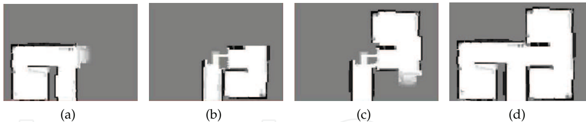
Fig. 3. Local maps acquired by individual robots (a-c) and global map merged by the server (d) from data of the environment illustrated in Figure 2.
