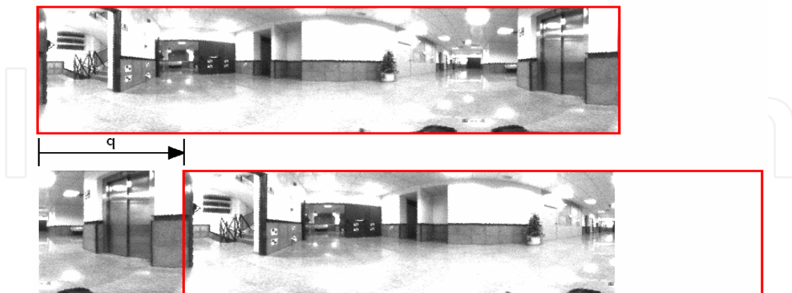
Fig. 3. Two panoramic images captured in the same point of the environment but with different heading for the robot.
