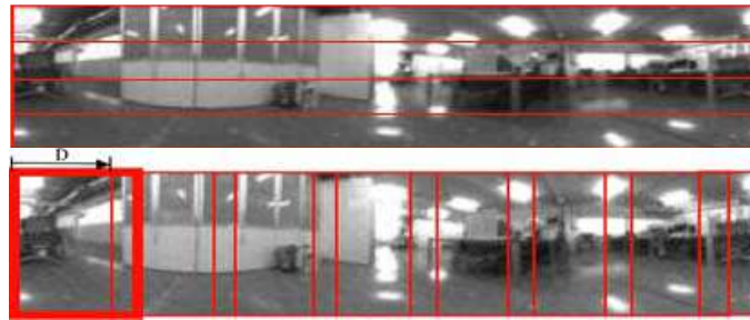
Fig. 4. Cells used to compute the current position and the orientation of the robot.
