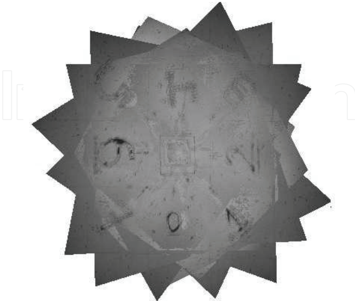
Fig. 11. Single-robot SLAM: generated map of the site
