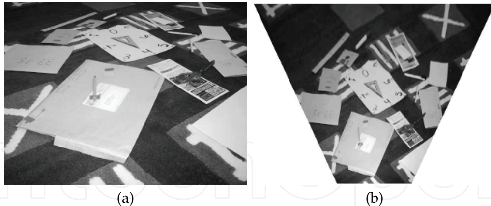
Fig. 2. Overhead view: (a) The image of a planar surface taken with tilt = 33^\circ , (b) The corresponding generated overhead view.
