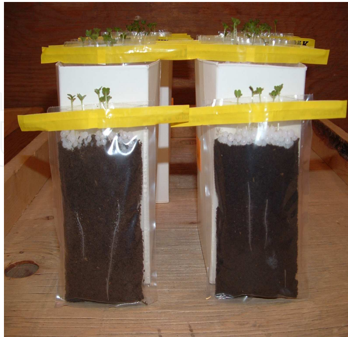
Fig. 1. Mustard root length bioassay performed in Whirl-Pak bags.
