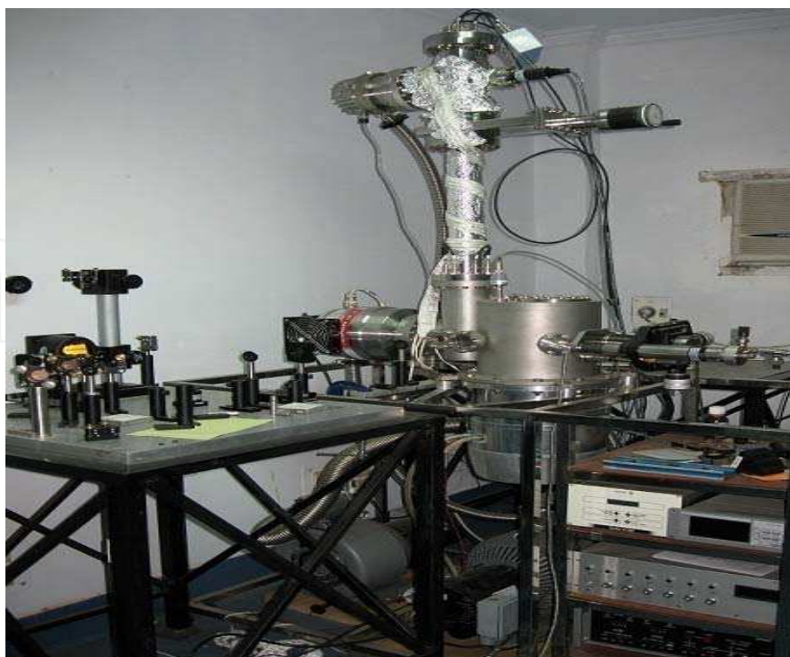
Fig. 9. Picture of our supersonic molecular beam linear time of flight mass spectrometer.
