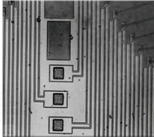
Fig. 13. LFPA thermo-electric detector with squared perimeter contact pixels
