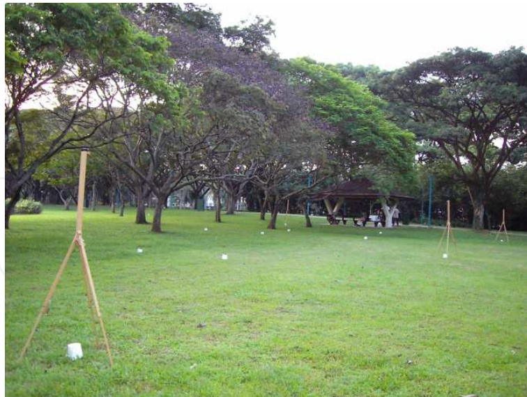
Fig. 13. ALS experiments in an obstacle ridden environment – the experiment was carried out in a 30m×30m region in a park with several trees in the region. Several of the sensors were placed behind trees, as seen in the picture.
