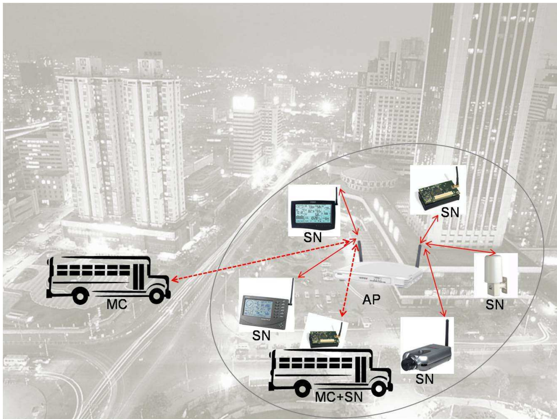
Fig. 1. Reference network topology for general I2V applications.
