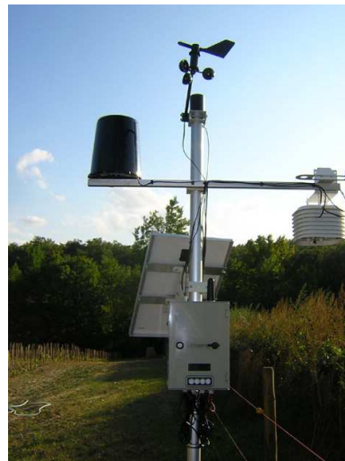
(b) VineSense GPRS Gateway with Weather Sensors
