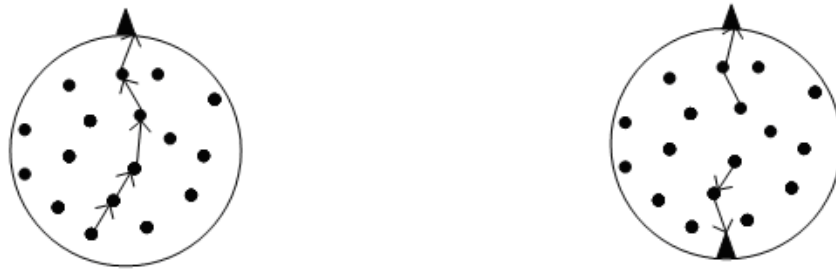
(a) A single base station on the periphery on a small scale WSN. (b) Two base stations on the periphery on a small scale WSN
