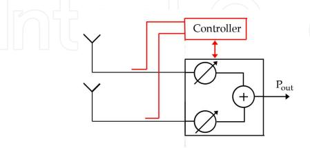
Fig. 2.3. Sketch of equal gain combining.
