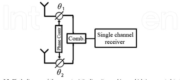
Fig 3.2. Block diagram of the opportunistic diversity combiner, which is connected to the receiver.
