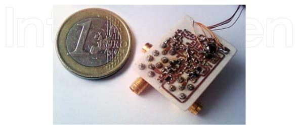
Fig. 3.4. Photo of the add-on diversity combiner, with SMA connectors for the two diversity antennas and the receiver.
