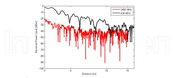
Fig. 1.4. Typical measurement at 434 MHz and 2450 MHz.
