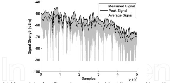
Fig. 3.6. Measured signal in office environment received from diversity combiner with peak and average signals marked.
