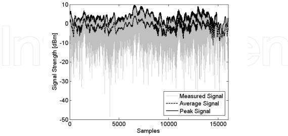
Fig. 3.5. Measured signal in reverberation chamber received from diversity combiner with peak and average signals marked.
