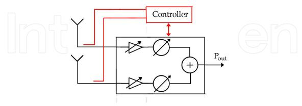
Fig. 2.4 Sketch of maximum ratio combining.
