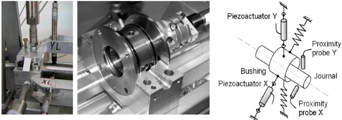
Fig. 1. Arrangement of the controllable journal bearing
