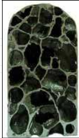
Fig. 8. TiH 2 foam sample obtained by cold uniaxial pressure
