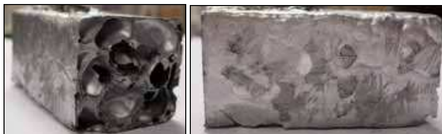
Fig. 9. Shaped MGI part with dense skin
