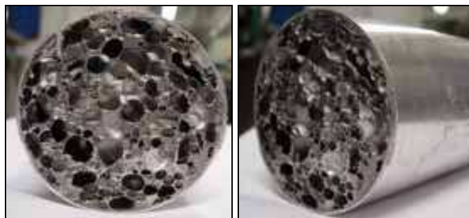
Fig. 11. MGI foam cores attached by mechanical bonding (front and lateral view)
