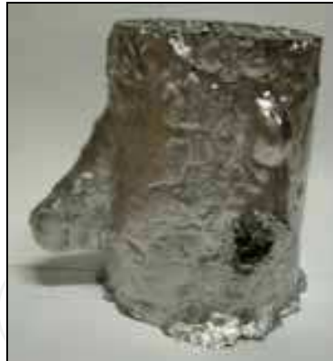
Fig. 10. MGI foam core insert with spacers
