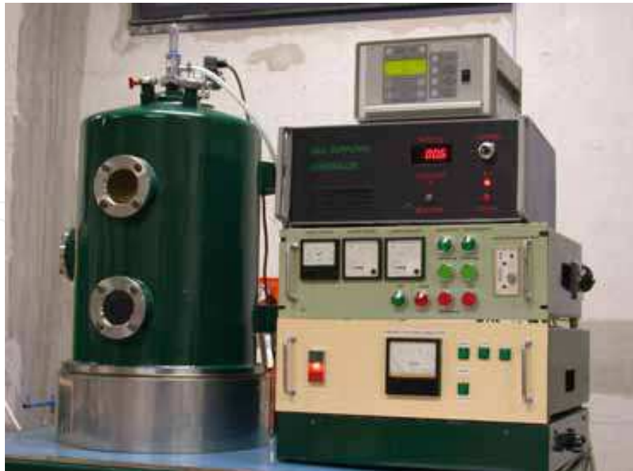
Fig. 1. The scheme of the system used for deposition of hard carbon coatings by PACVD method
