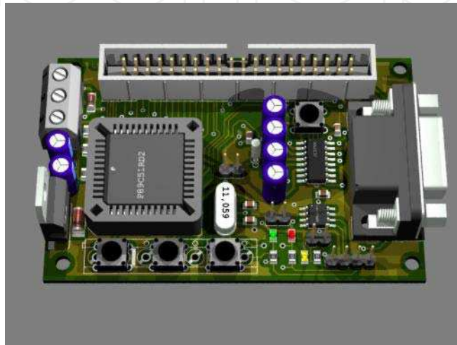
Fig. 3. Example of 3D Model generated from 3DEagle plug-in.
