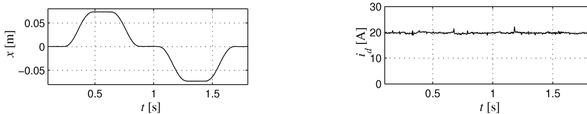
Fig. 11. Trajectories of position x and current i_d measured on the experimental system in the case of kinematic control
