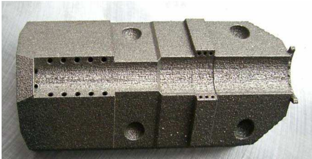
Fig. 14. Laser sintered upper component of the jig
