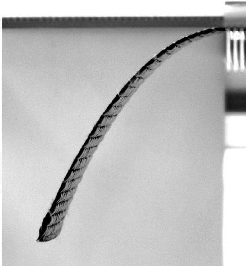
Fig. 10. Cantilever bending test
