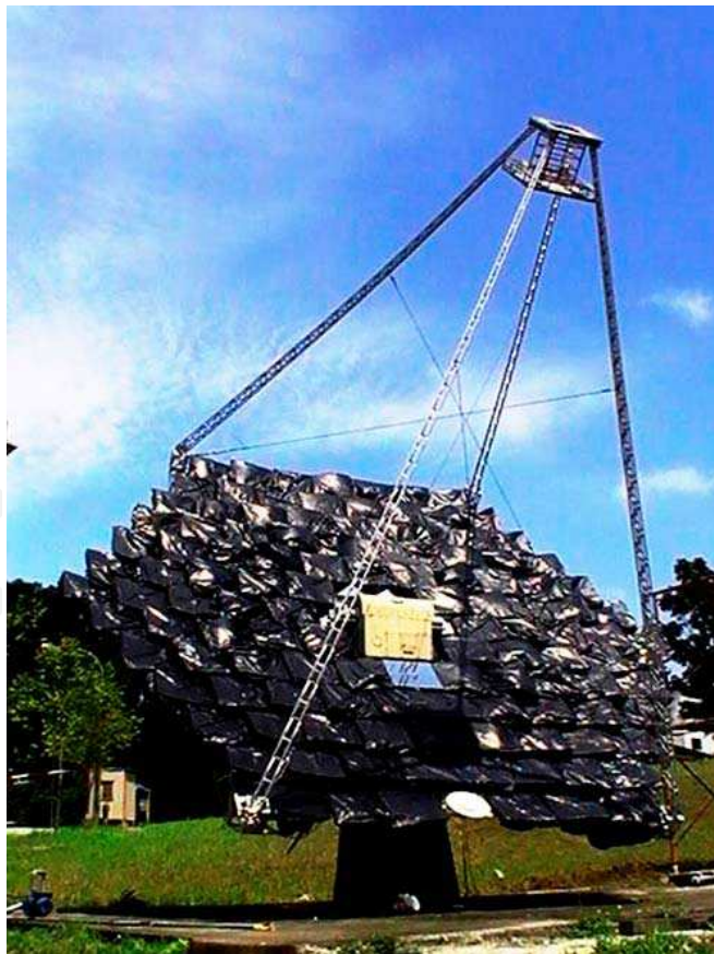
Fig. 9. A prototype of 25\text{m}^2 on-axis Non-Imaging Planar Concentrator (NIPC) that has been constructed at Universiti Tunku Abdul Rahman (UTAR)
