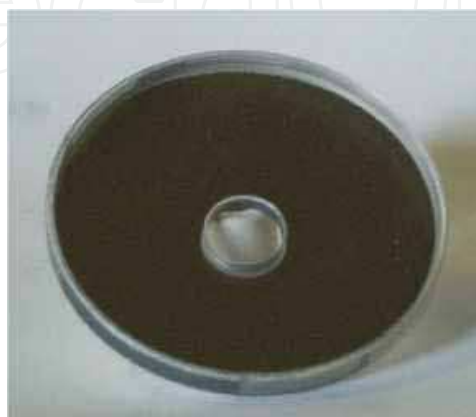
Fig. 5. Collector A1 (Mangin60) realized in glass.
