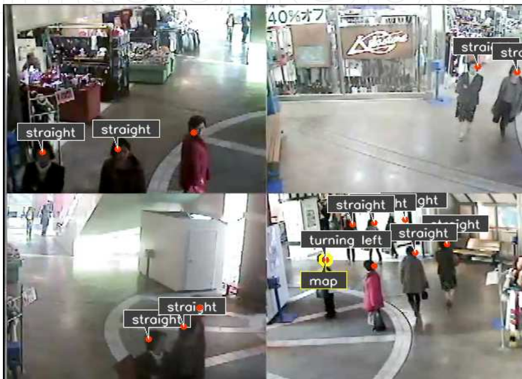
Fig. 7. Primitive recognition results. The box above a person indicates the detected local behavioral primitive (style of walking) and the one below shows the spatial primitive.
