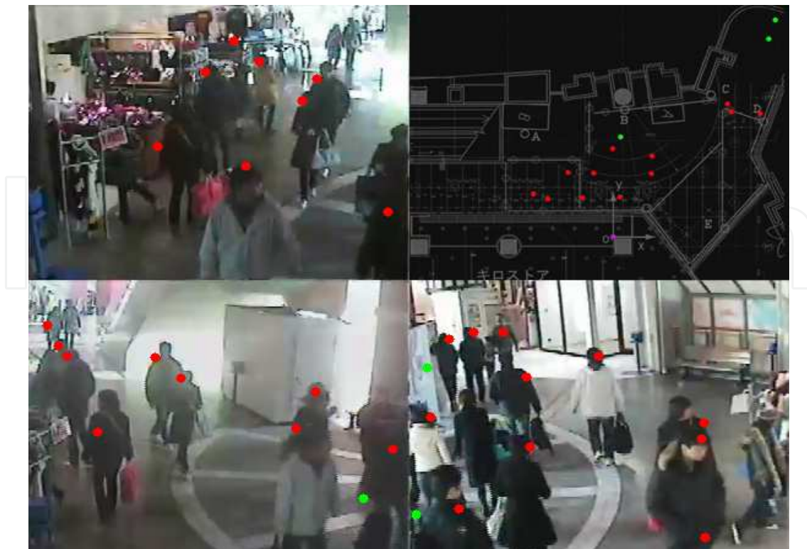
Fig. 6. Example of the integrated position estimation. The red dots show the head estimation results and the green dots show the torso estimation where head was not detected or when person was out of camera tracking area.
