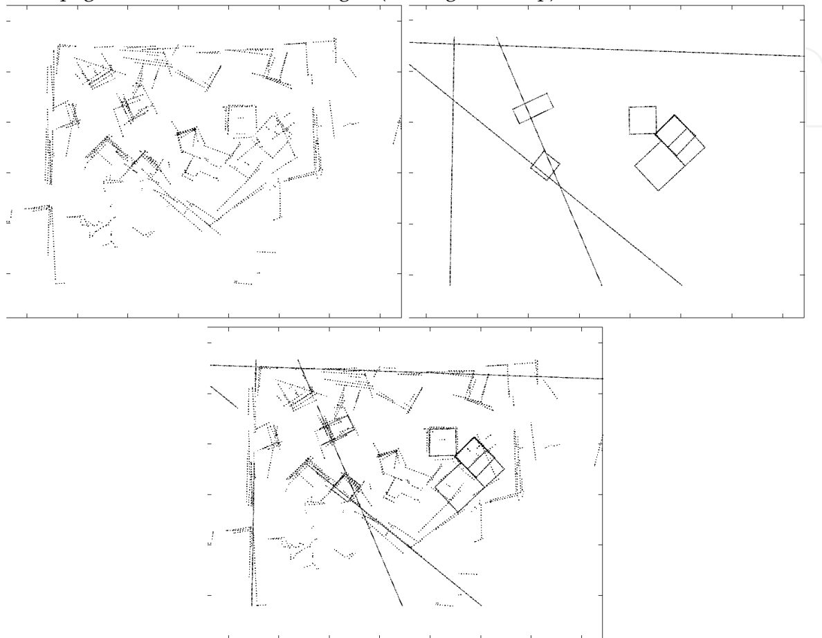
Fig. 8. Virtual Scans in an early stage of FFS. a) global map b) the Virtual Scan consisting of points representing detected lines and rectangles c) superimposition of real data and Virtual Scan. This is the data used in the next FFS iteration.
