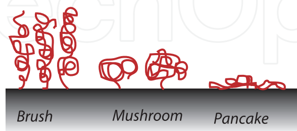
Fig. 1. Possible polymer conformations, depending on quality of solvent, polymer degree of ionization and grafting distance.
