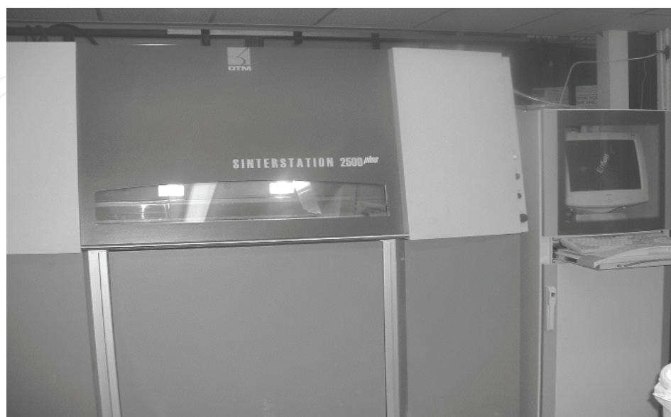
Fig. 4. The SLS Sintersation 2000 apparatus (Courtesy of CRDM)
