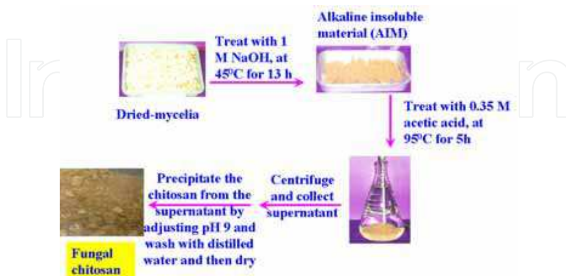
Fig. 2. Extraction of chitosan from mycelia of fungus G.butleri grown in solid substrate fermentation
