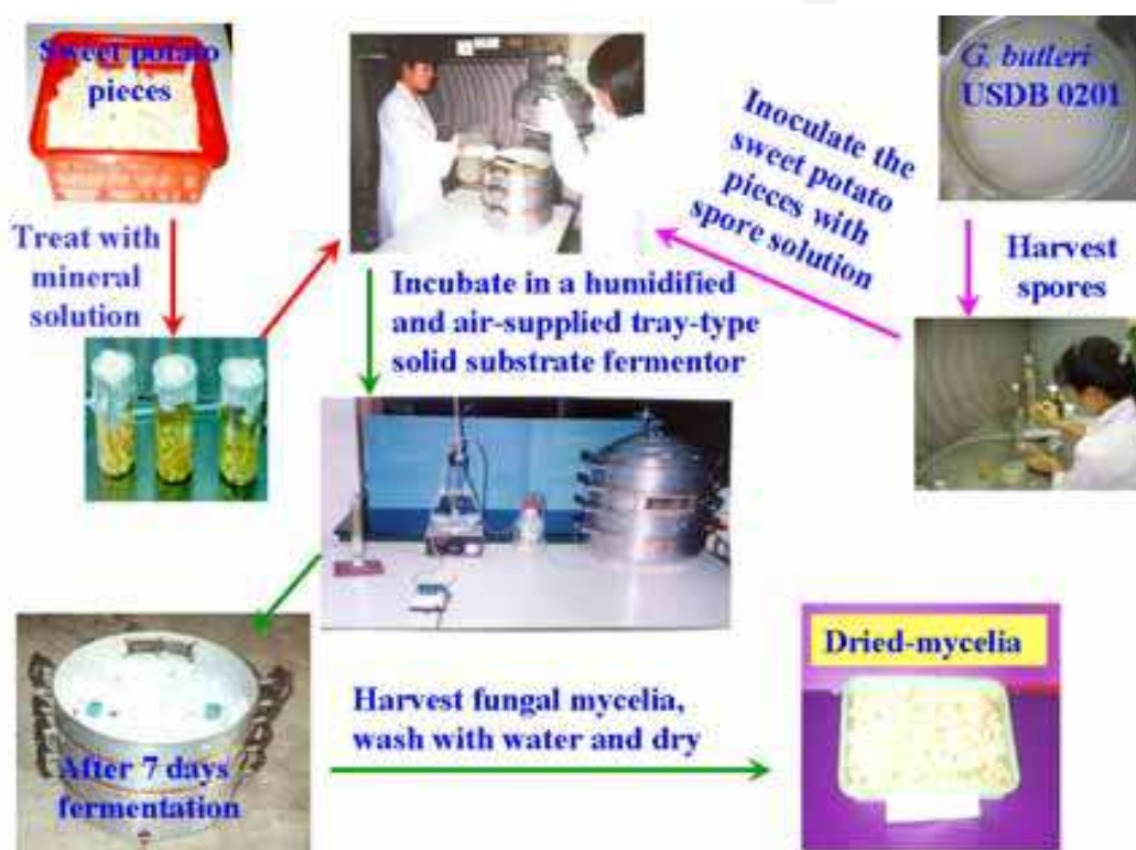
Fig. 1. Fungus Gongronella butleri USDB 0201 was grown on sweet potato pieces in a tray-type solid substrate fermentor. Sweet potato pieces were used as solid support and as carbon source. The dried fungal mycelia were used to extract chitosan.
