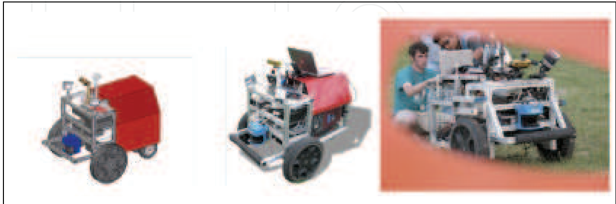
Fig. 4. 'Bearcat Cub' intelligent vehicle designed for the Intelligent Ground Vehicle Contest
