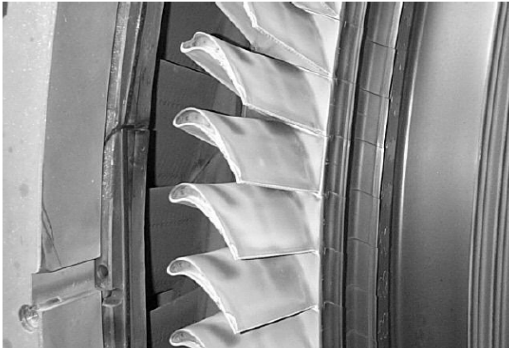
Fig. 3.3. Typical turbine stage. [From Shepherd, D.G., Introduction to the Gas Turbine, D. Van Nostrand Co., Inc.
