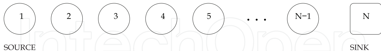
Fig. 1. Linear multihop path between the source node and the destination sink.
